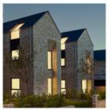
Eaves rooflight with vertical window top-lighting stair
